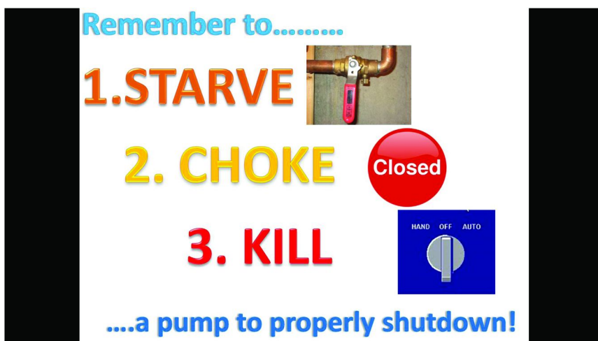
Figure 3. Safe Process Pump Shutdown
